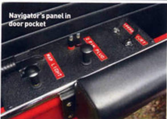
Red Dymo tape and flick switches, works spec
