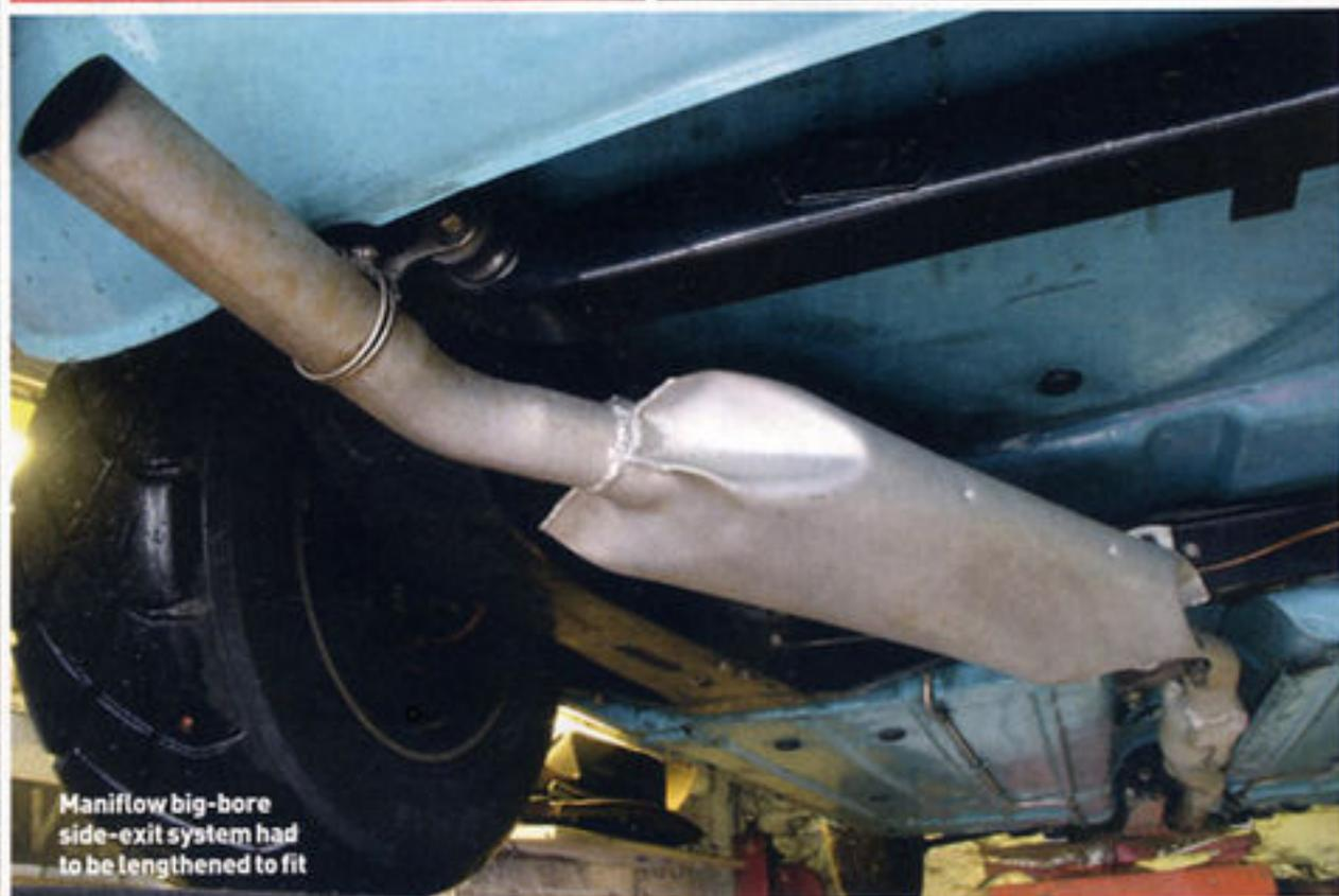
Manifold big-bore side-exit system had to be lengthened to fit
