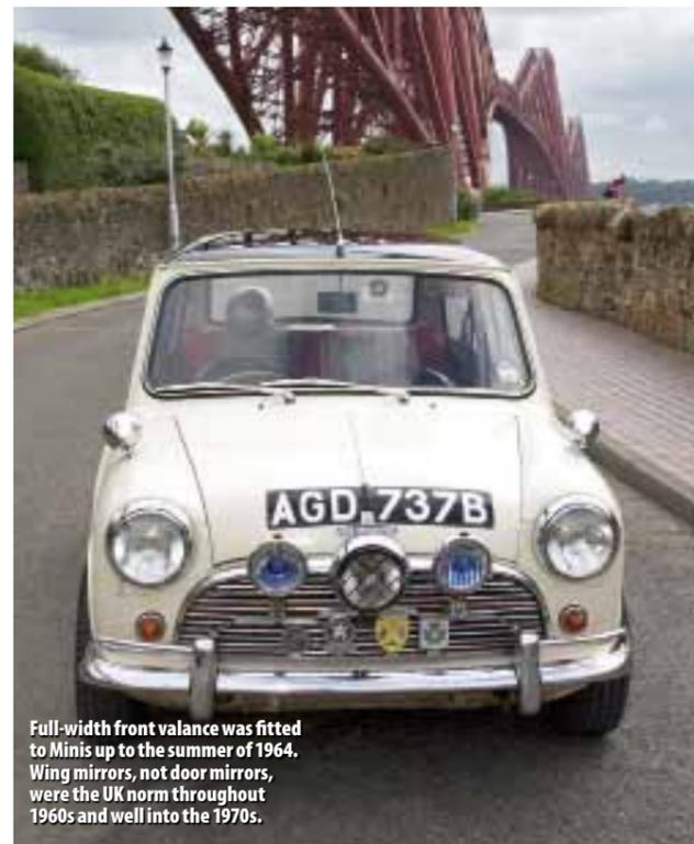
Full-width front valance was fitted to Minis up to the summer of 1964. Wing mirrors, not door mirrors, were the UK norm throughout 1960s and well into the 1970s.
