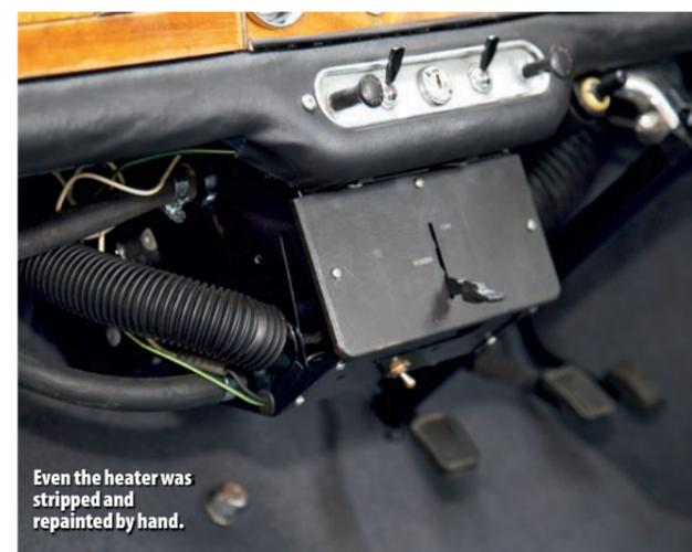
Even the heater was stripped and repainted by hand.
