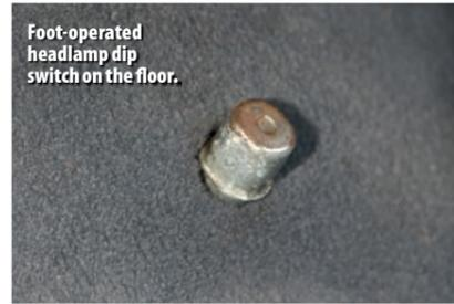
Foot-operated headlamp dip switch on the floor.
