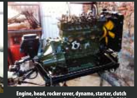
Engine, head, rocker cover, dynamo, starter, clutch slave and thermostat housing were originally BMC green. Some of these components have been left unpainted for serviceability. Standard fan would have been a 16-blade steel item.
