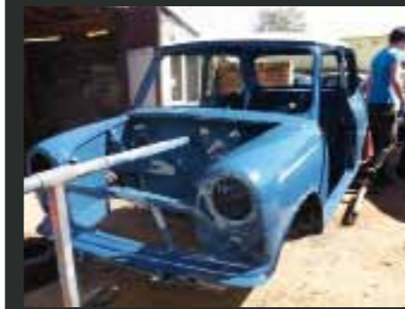
A very Scottish colour scheme and spot-on for the Mk1 Cooper range. The diagonal panel stiffener in the front panel would usually be painted black to hide it from view. Reassembly took only two weeks.
