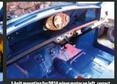
3-bolt mounting for DR3A wiper motor on left, correct rectangular headlamp dip switch above tunnel. Coopers never had floor starter switch. Mk1 Cooper floorpan had lesser models' wandshift aperture blanked and covered with mastic at the factory.
